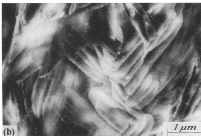
Fig. 3 AFM of HDPE A on the top surface of oriented iPP film and B on the top surface of freshly cleaved mica. The samples were heat-treated at 150°C for 15 min and then quickly cooled to room temperature. Arrow, molecular directions of oriented iPP substrate in A
